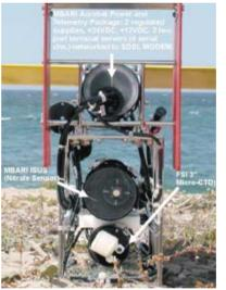
The power and telemetry system components are contained within a 4.5 inch diameter Aluminum pressure housing measuring 12 inches in length and mounted directly behind the Acrobat motor controller. Two printed circuit boards, mounted inside, were developed. The first converts the incoming AC power into the two principle DC supplies used by the various systems, while the second supports the embedded terminal servers and provides RS232 and RS485 level shifting.
