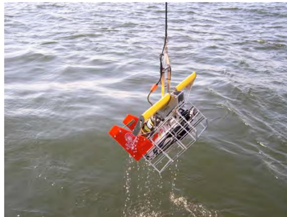
Figure 4. Acrobat vehicle being recovered on R/V Pelican during April 2009 MCH cruise M13.
