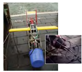
Figure 2. Towed Undulating Vehicle (Acrobat) with Microstructure Instrument (TOMASI).
