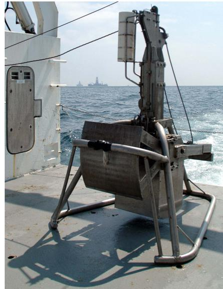
Figure 3: 2500  $\text{cm}^2$  box corer aboard R/V Pelican in vicinity of Deepwater Horizon well site in the background.
